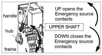
Figure 1-7. Emergency (upper shaft) operation on 150–600 amp. J–design transfer switches.
